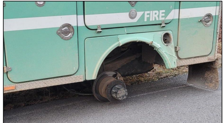
Image shows the driver's side wheel studs that were sheared off.
